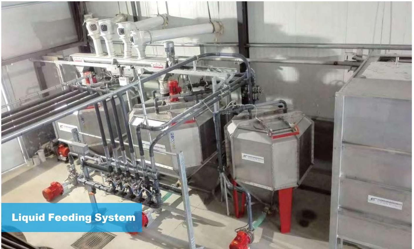
*Liquid feeding was, in fact, the most traditional way of pig feeding adopted from their natural habit. However, the technical standard for liquid feeding was behind the steps of modernized pig breeding, and thus many modern large scale pig farms chose to use the dry feed system. With the development and application of intelligent management and automatic liquid feeding technologies, liquid feeding system is becoming the new fashion.*
